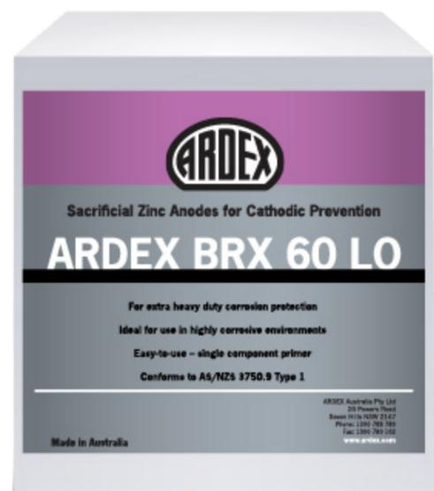
ARDEX BRX 60 LO Low Output Anodes are for use within concrete where repairs due to reinforcement corrosion are required. The anodes provide cathodic prevention to incipient anodes (halo effect) or corrosion control to limit corrosion rates of corroding bars embedded in original concrete. It is recommended for use in conjunction with the ARDEX BR Repair Mortar Range for ultimate corrosion prevention.
