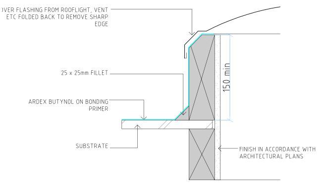
NOTE: 1/ For maximum penetration size of 1200x1200mm 2/ External corners to be formed as shown
