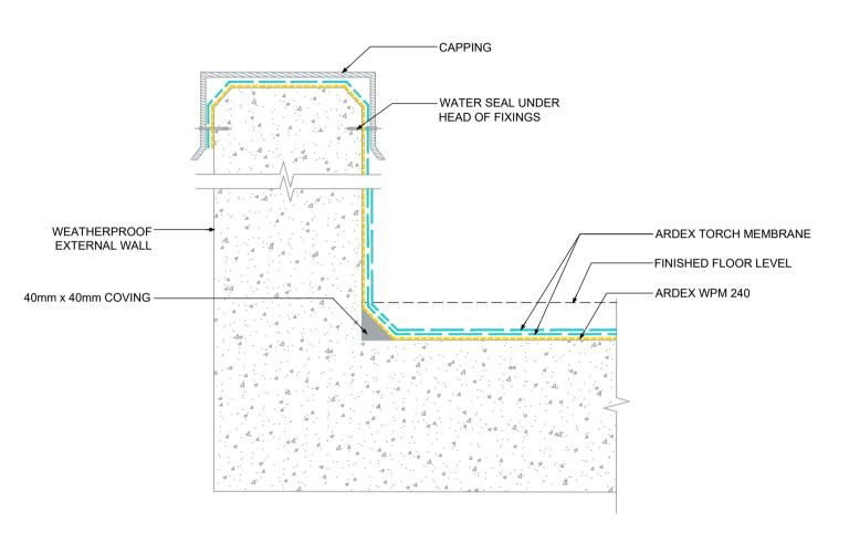
PARAPET WALL CAPPING DETAIL - TORCH APPLIED MEMBRANE
