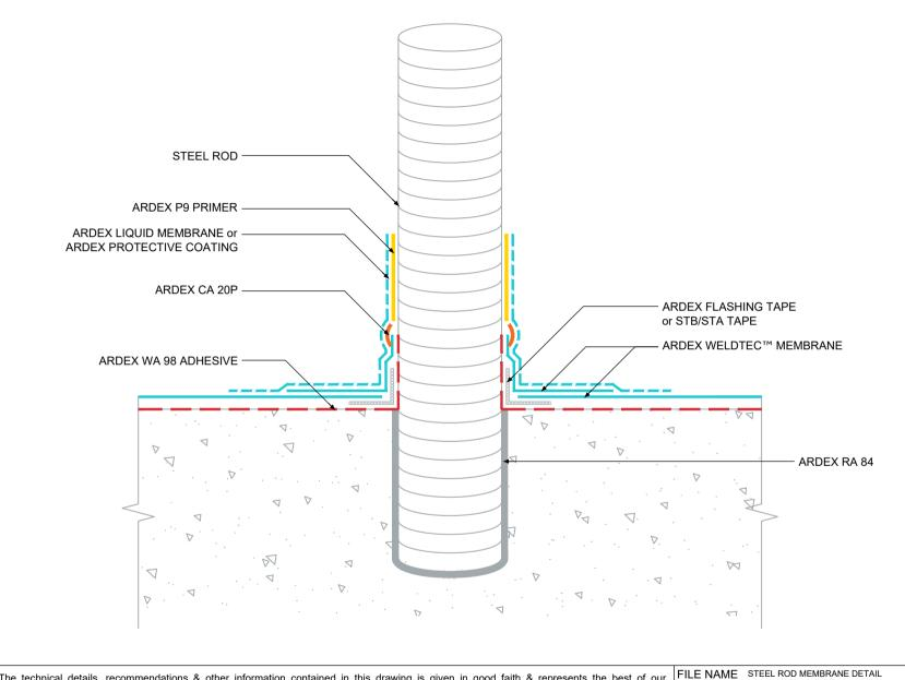
STEEL ROD MEMBRANE DETAIL OPTION 1 - ARDEX WELDTEC™
