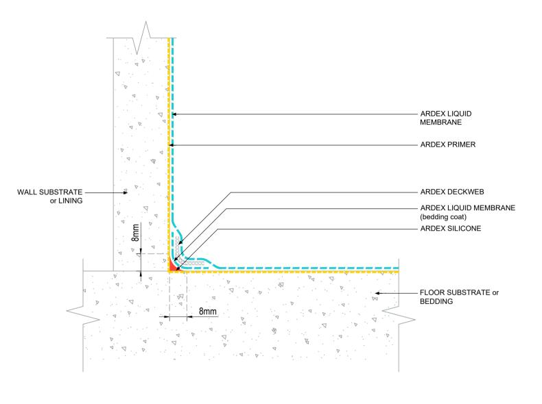
TYPICAL FLOOR TO WALL TRANSITION DETAIL -ARDEX SILICONE & ARDEX DECKWEB
