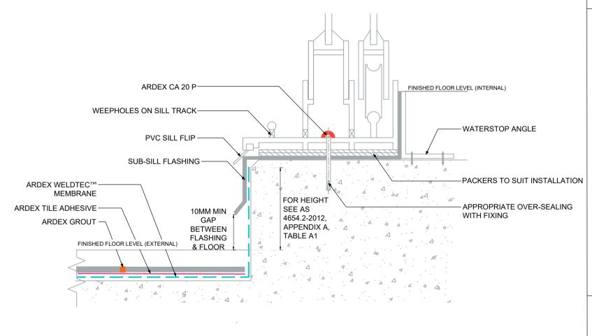
TERMINATION AT EXTERNAL DOOR OPENING HIGHER THAN SILL UPWARD TERMINATION - ARDEX WELDTEC MEMBRANE
