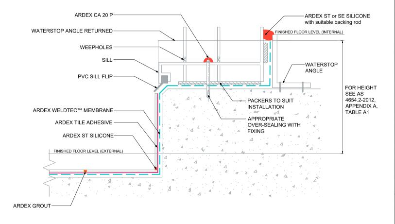
TERMINATION AT EXTERNAL DOOR OPENINGS NO SUB SILL -ARDEX WELDTEC MEMBRANE
