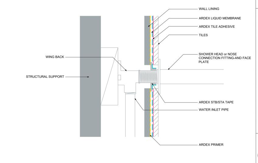
TYPICAL SHOWER TO HEAD OR FLEXIBLE HOSE CONNECTION - LIQUID MEMBRANE WITH ARDEX STB/STA TAPE
