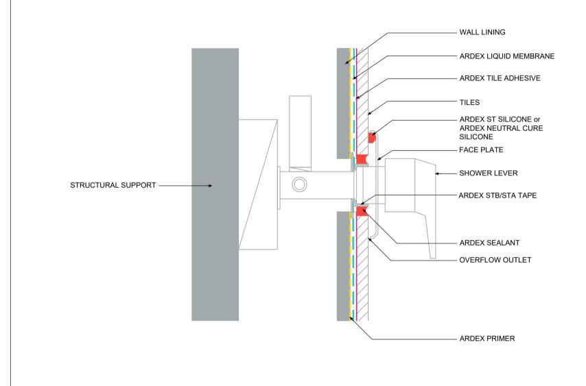
TYPICAL SHOWER MIXER USING ARDEX SEALANT WITH ARDEX STB/STA TAPE
