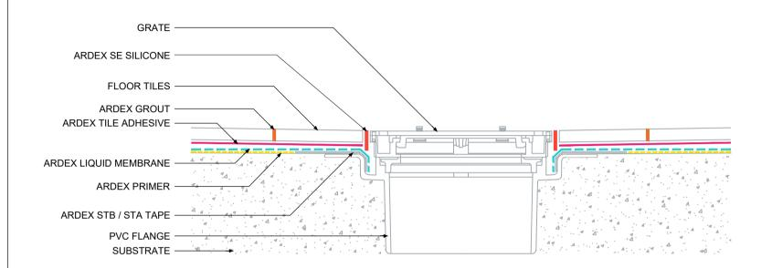
DRAINAGE FLANGE WATERPROOFING WITH ARDEX LIQUID MEMBRANE AND ARDEX STB/STA TAPE
