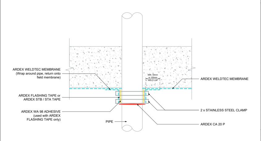
HORIZONTAL PIPE PENETRATION WITH ARDEX WELDTEC MEMBRANE (PRE-APPLIED)
