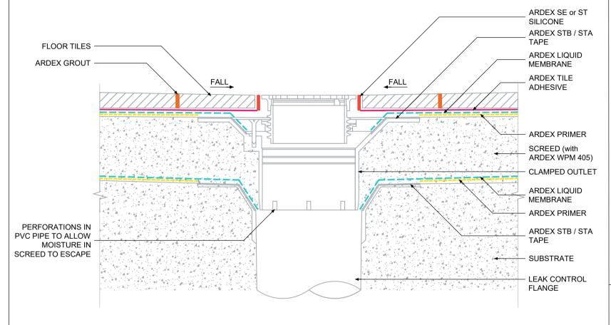
INTERNAL CLAMP DOWN WASTE OUTLET DETAIL -DUAL MEMBRANE SOLUTION WITH ARDEX LIQUID MEMBRANE
