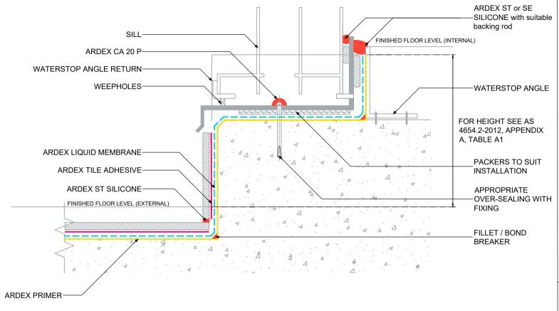
TERMINATION AT EXTERNAL DOOR OPENINGS - ARDEX LIQUID MEMBRANE
