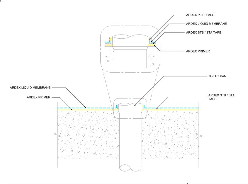
TOILET PAN TERMINATION WITH ARDEX LIQUID MEMBRANE
