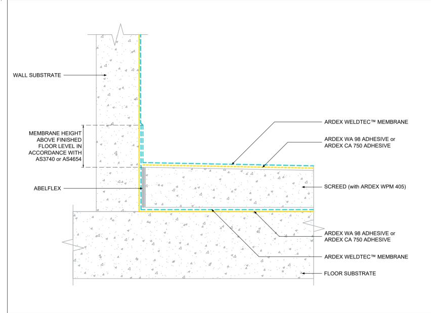
TYPICAL FLOOR TO WALL TRANSITION DETAIL - DUAL MEMBRANE SOLUTION WITH ARDEX WELDTEC MEMBRANE
