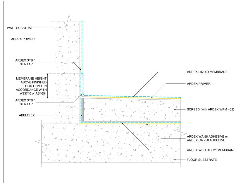
TYPICAL FLOOR TO WALL TRANSITION DETAIL - DUAL MEMBRANE SOLUTION WITH ARDEX WELDTEC & LIQUID MEMBRANE
