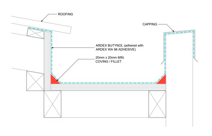
ROOFTOP GUTTER WITH PARAPET DOWNTURN
