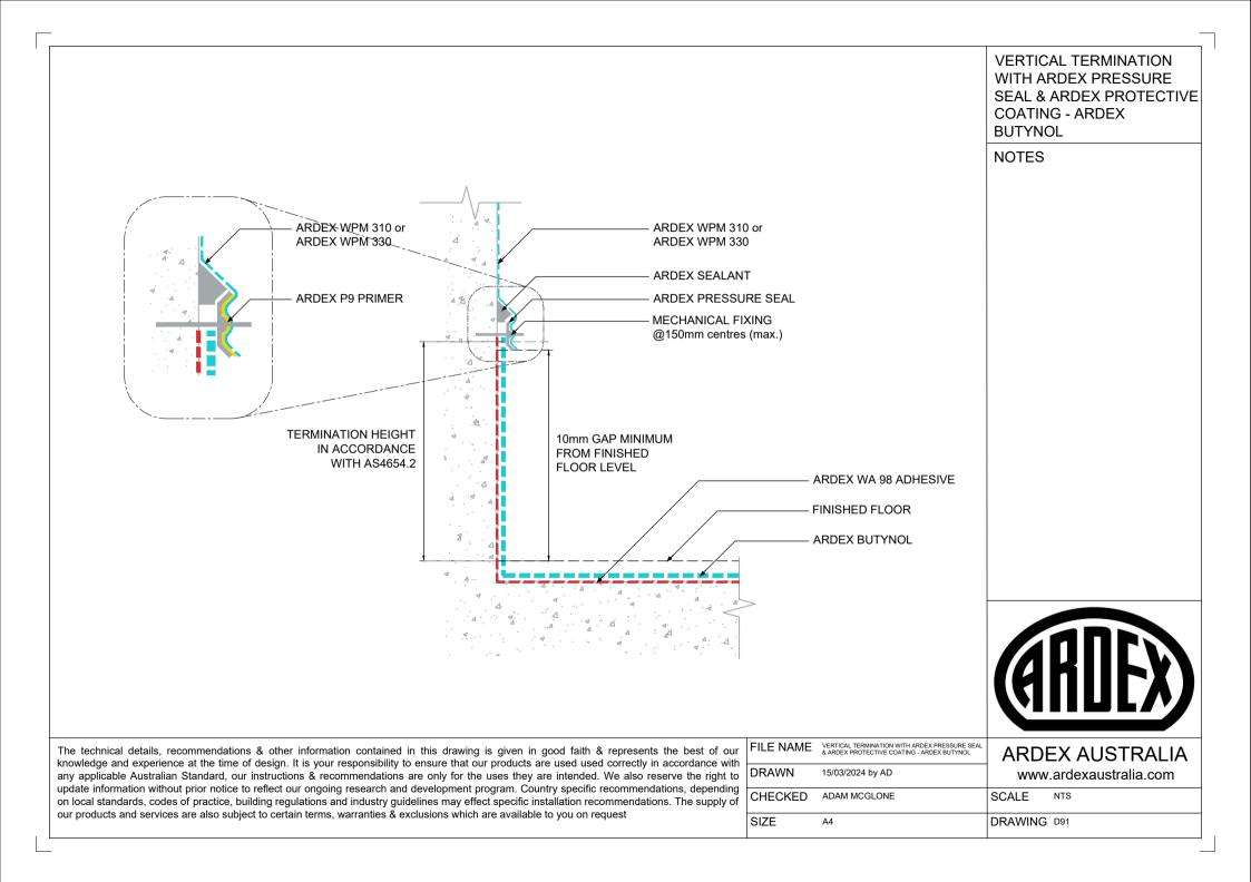
VERTICAL TERMINATION WITH ARDEX PRESSURE SEAL - ARDEX BUTYNOL
