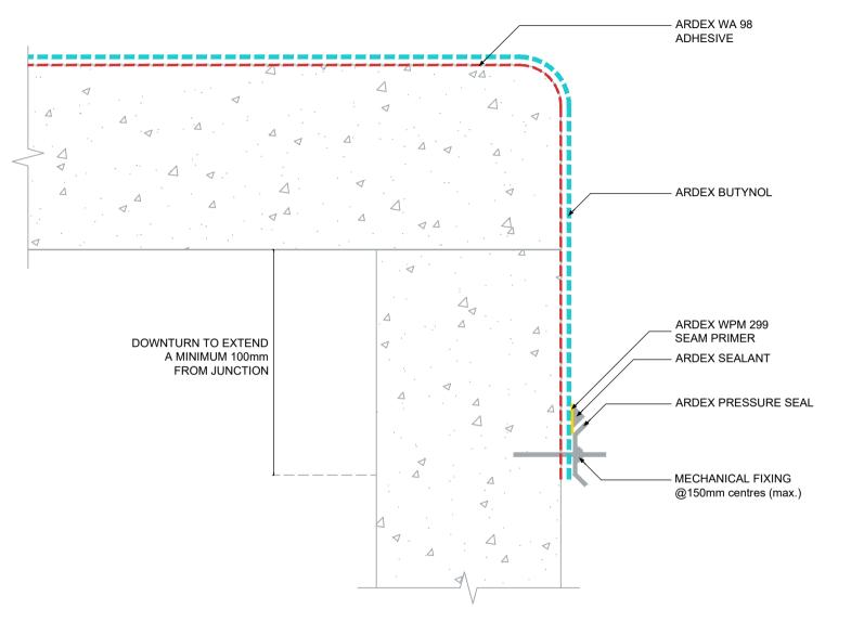
VERTICAL DOWNTURN TERMINATION WITH ARDEX PRESSURE SEAL - ARDEX BUTYNOL
