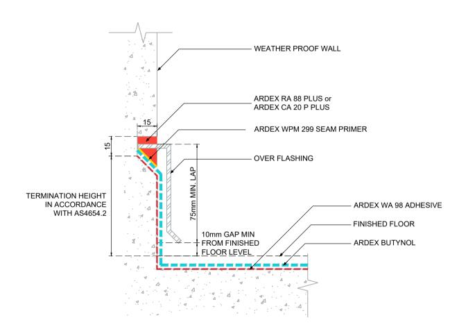
VERTICAL OVER - FLASHING TERMINATION WITH MEMBRANE INTO REGLET -ARDEX BUTYNOL
