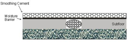
As per steps 26-27, the joint has been cleaned and filled with a backer rod. The Moisture Barrier has
