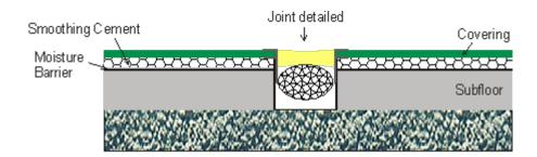
As per step 30 Moisture Barrier is painted thoroughly down into the joint. A suitable flexible sealant system is then installed (may include mouldings or metal extrusions
