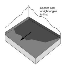
The coats are applied at 90-degree angles to obtain a complete coverage
