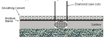
As per step 28, when underlayment is fully cured, it is saw cut through to the FULL WIDTH of the JOINT
